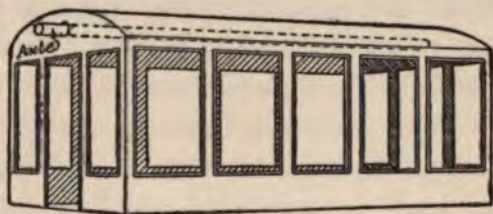
FIG. 159. — A Completed Car for the Ferris Wheel.
